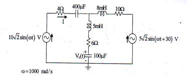
2- For the following circuit, if the switch is opened at t = 0 and after one second the switch is re-closed. Find  $V_o(t)$  and then use MATLAB to plot  $V_o(t)$  for the time interval  $0 \le t \ge 5 s$  (7 Marks)
