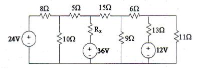
2. Use nodal analysis to solve for the nodal voltages for the circuit shown. Solve the equations using MATLAB. (4 Marks)
